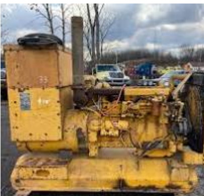
Figure Caterpillar D333-155KW Diesel Generator
