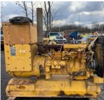
Figure Caterpillar D333-155KW Diesel Generator
