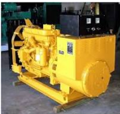
Figure Caterpillar -D333 Generator Set
