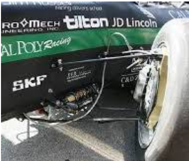
Figure 1: Broken Suspension Components
