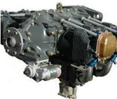
Figure Lycoming O235-L2C Engine
